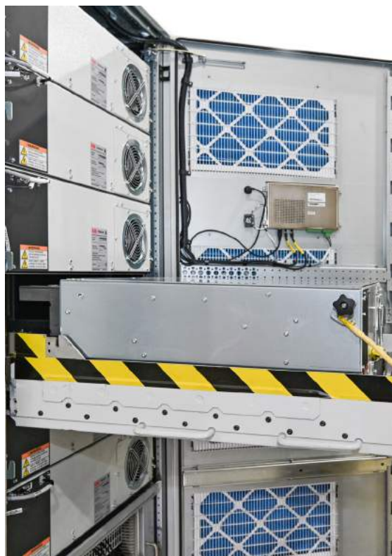
03. Power Electronics Building Block (PEBB)
